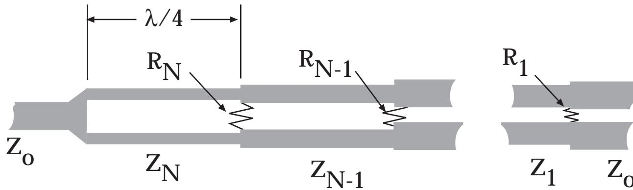
Note that for this figure and the following calculations the numbering of the sections has been reversed, and that all sections are  $\lambda/4$  long.
